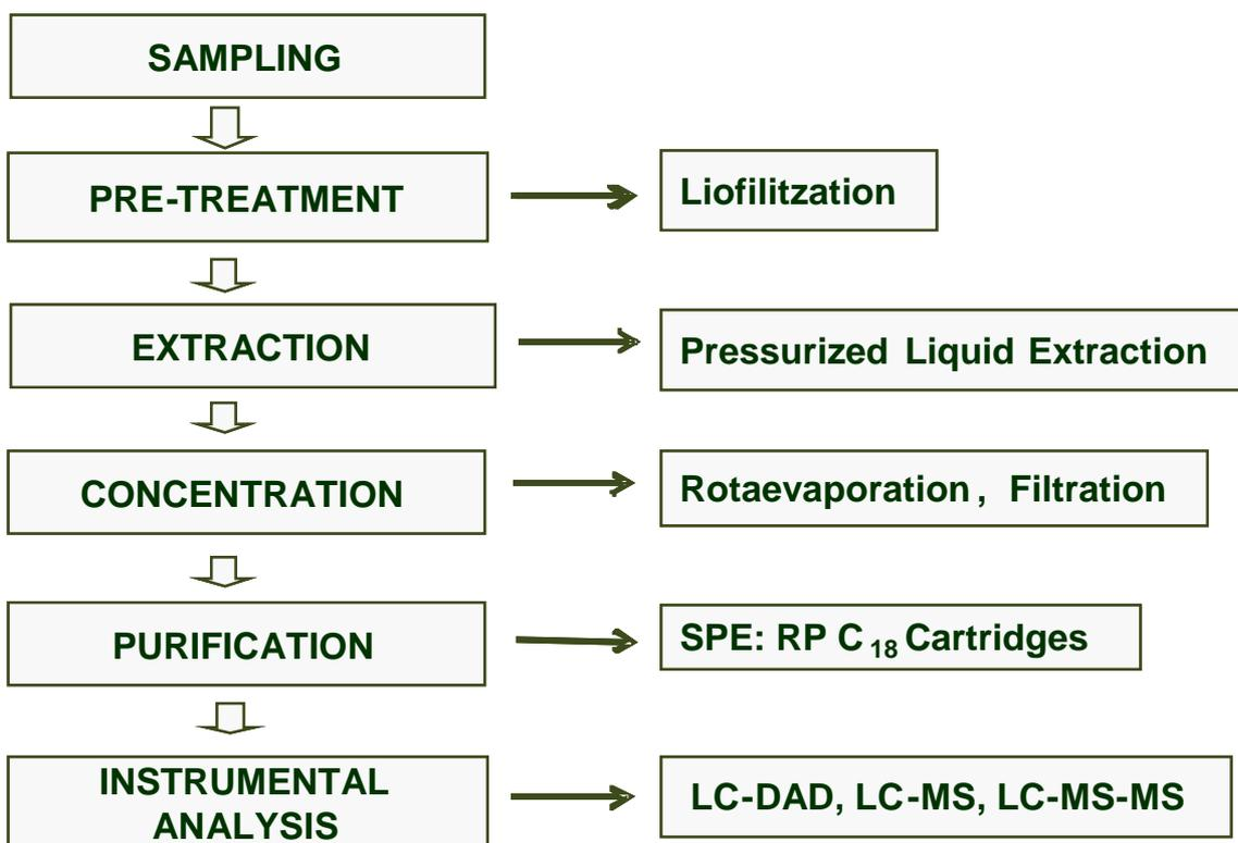
Figure 2. Sample preparation steps for the determination of benzoxazinones and further degradation products in plants and soils
